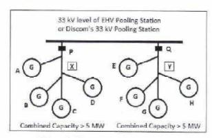
In this case, Generators 'A' to 'D' and 'E' to 'H' are connected to a Pooling Sub-Station of STU or Discom through separate & dedicated feeders having separate inter-connection points at 'P' and 'Q' respectively.
