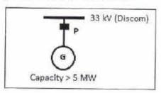
In this case, the Forecasting shall be provided by the QCA at Point 'P'. Scheduling and Accounting shall be done by MSLDC at Point 'P'.
