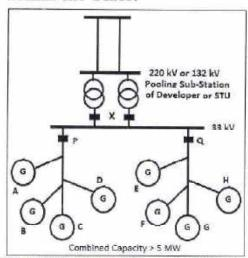
In this case, a group of generators ('A' to 'H') are connected at 33 kV level of the EHV Pooling Sub-Station through common 33 kV feeders.
