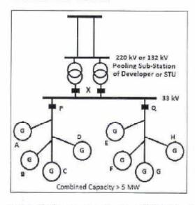
In this case, multiple generators ('A' to 'D') are connected at 33 kV level of the EHV Pooling Sub-Station through common 33 kV feeders selling power within the State.
